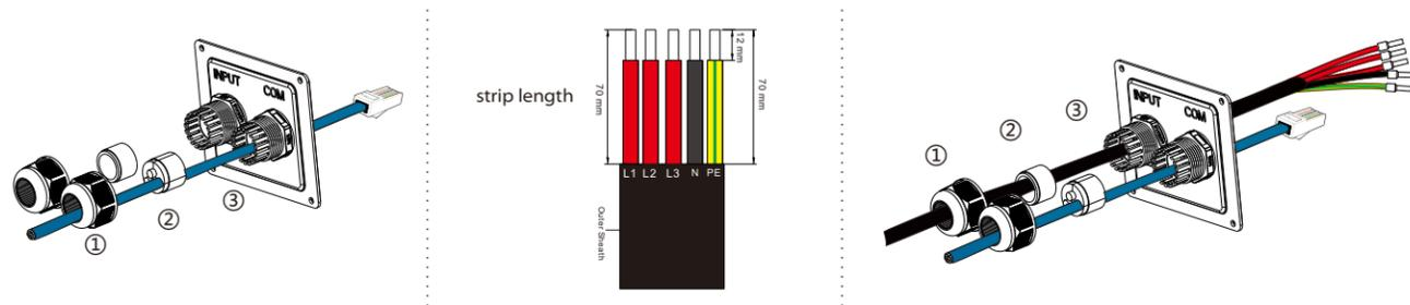
STEP 9: Insert the wires into the terminal blocks, then block the terminal with the straight screwdriver.
