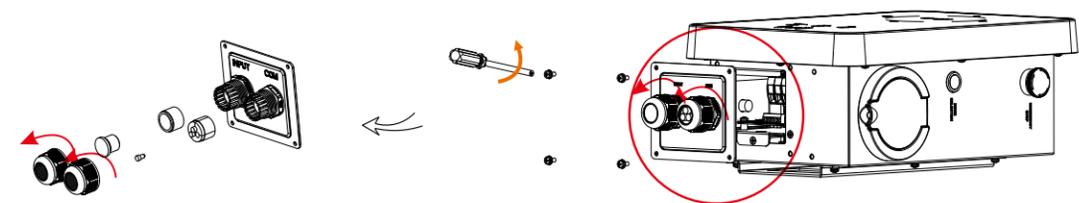
STEP 5: Unscrew the countersunk screw of the base plate of communication board with the cross screwdriver. Then pull the base plate of communication board out .
