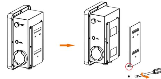
STEP 2: Fix the back bracket and the cable hook (only for type P) to the wall.
