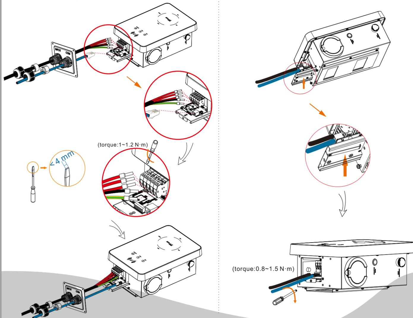
STEP 11: Push the rear cover to appropriate position of the cables and screw the self tapping screws with the cross screwdriver. Then tighten the waterproof fastening head.
